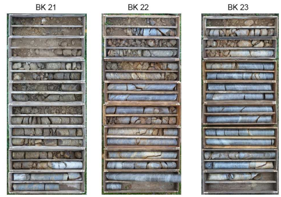
Figure 4. Drilling cores of three drillings (0 – 16 m) indicating stable rocky underground to define one radio telescope location. Each box corresponds to one meter depth from surface (most upper box) to –16 m (bottom box).
